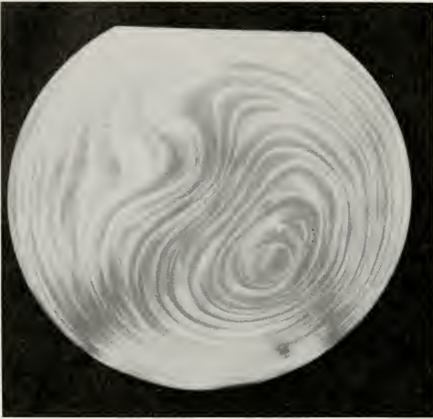
Fig. 9 Concentration-enhanced oxidation, showing dopant variations in a heavily doped phosphorus substrate.
