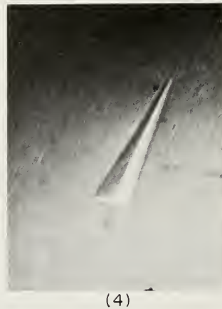
Fig. 21 Common defects occurring in epitaxial layers. (a) Schematic representation of line (or edge) dislocation initially present in the substrate and extending into the epitaxial layer (item 1), an epitaxial stacking fault nucleated by an impurity precipitate on the substrate surface (item 2), an impurity precipitate caused by epitaxial process continuation (item 3), growth hillock (item 4), and bulk stacking faults one of which intersects the substrate surface thereby being extended into the layer (item 5). (b) Photographs of defects in actual wafers. Dislocations revealed as circular etch pits by Secco etching in a region of slip on a \langle 100 \rangle wafer (item 1), epitaxial stacking faults on a \langle 100 \rangle wafer (item 2), dislocations revealed by Sirtl etching in a \langle 111 \rangle wafer (item 3), and a growth hillock on a \langle 111 \rangle wafer, visible without etching (item 4).
