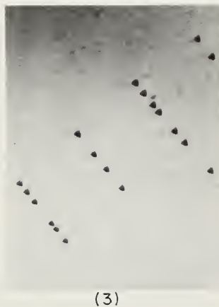
Fig. 21 Common defects occurring in epitaxial layers. (a) Schematic representation of line (or edge) dislocation initially present in the substrate and extending into the epitaxial layer (item 1), an epitaxial stacking fault nucleated by an impurity precipitate on the substrate surface (item 2), an impurity precipitate caused by epitaxial process continuation (item 3), growth hillock (item 4), and bulk stacking faults one of which intersects the substrate surface thereby being extended into the layer (item 5). (b) Photographs of defects in actual wafers. Dislocations revealed as circular etch pits by Secco etching in a region of slip on a \langle 100 \rangle wafer (item 1), epitaxial stacking faults on a \langle 100 \rangle wafer (item 2), dislocations revealed by Sirtl etching in a \langle 111 \rangle wafer (item 3), and a growth hillock on a \langle 111 \rangle wafer, visible without etching (item 4).
