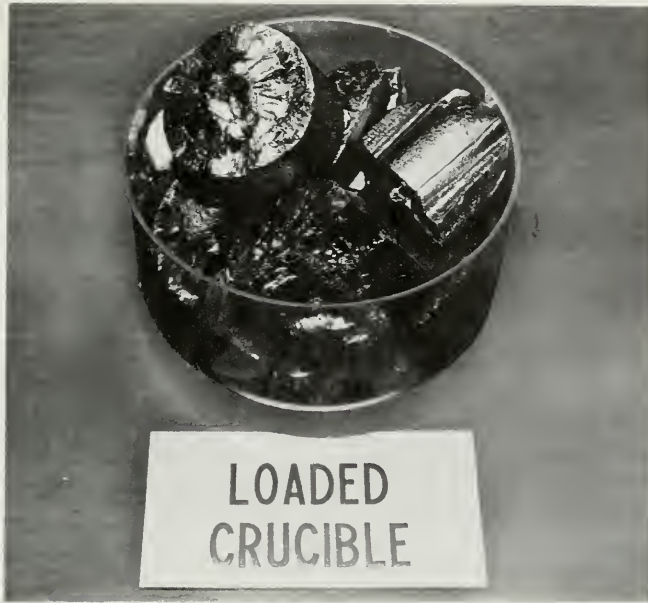
Fig. 3 EGS in chunk form loaded into a quartz crucible.
