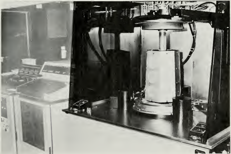
Fig. 13 A radiant-heated barrel reactor.
